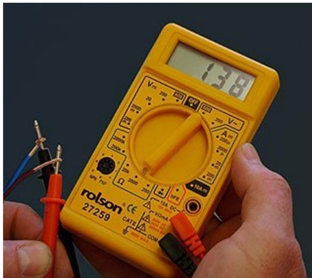
Measuring resistance of a heater
