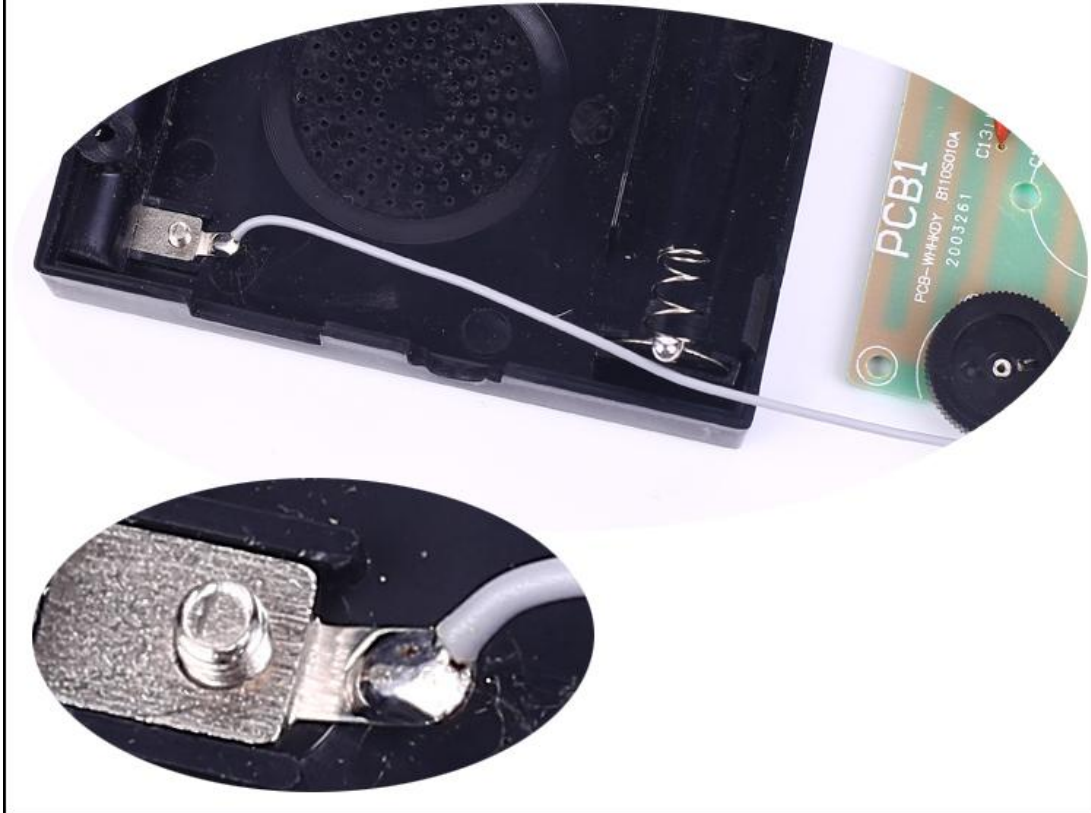
Step 37: Connect 120mm Gray Antenna Wire to Antenna Metal Sheet.
