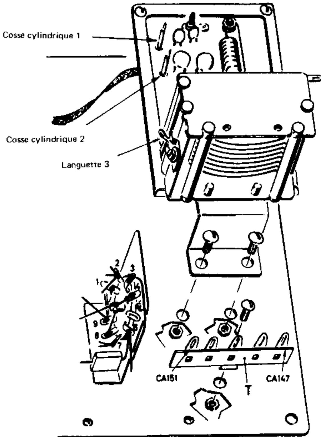
FIXATION DE LA BARRETTE T ET DU BLOC FM SUR LE CHASSIS
